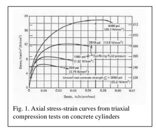
Figure 1, as shown in Reinforced Concrete Structures <sup>3</sup> by Park and Paulay, page 20, Figure 2.11, axial compressive strength is increased 500% and ultimate strain is increased by 300% when confined by the fluid pressure.
