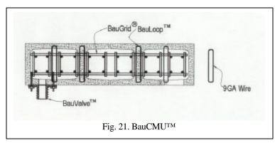
earthquake repair costs less than buildings constructed with conventional cast-in-place concrete structural systems. Ductile inelastic deformability of the BauCMU<sup>TM</sup> System without significant damage, is based upon a design of the frames and shearwalls using a BauBlock<sup>TM</sup> which is a standard double open end block modified to accept horizontal BauLadders® at 10 cm (4") on center. The special BauFlexmortar<sup>TM</sup> is designed to allow the BauBlock<sup>TM</sup> to
