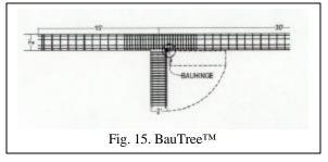
Frames of column-beam cages can be rapidly assembled to make BauTrees<sup>TM</sup>. Single-story or two-story BauTrees<sup>TM</sup> can be quickly set in place as one piece. A BauHinge<sup>TM</sup> attached at the top of the column BauCages<sup>®</sup> to the beam BauCage<sup>®</sup> will allow the BauTrees<sup>TM</sup> to be shipped from the plant as one piece without column rebar. At the site the column BauCages<sup>®</sup> will be rotated into position and then the column rebar charged. The
